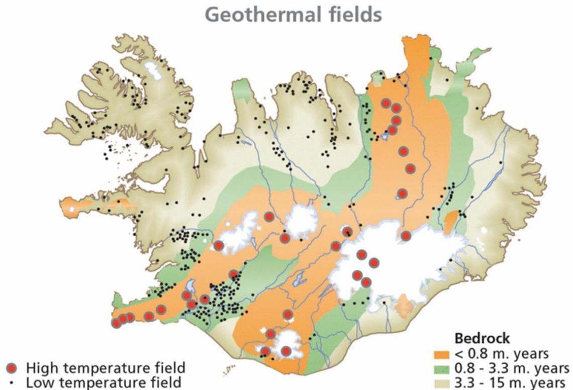
Figure 1: Geothermal fields of Iceland
