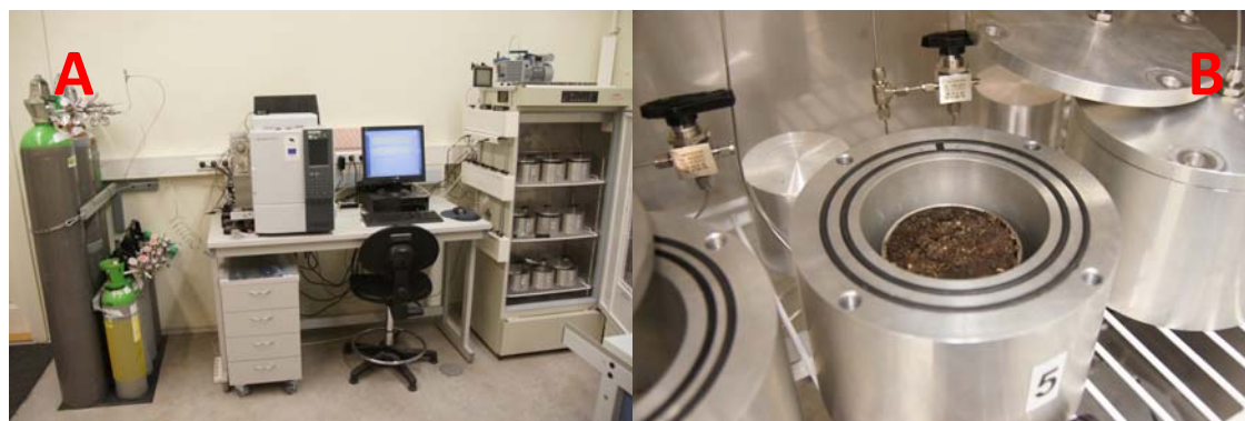
Figure 2. The measuring system (A) and the incubation vessel (B) to simultaneously quantify N 2 emissions from intact soil cores.
